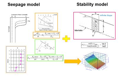
Fig. 11. Infiltration and Slope stability Analysis[19]
