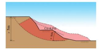
Fig. 3. Graphical representation of slope failure in cut slope
