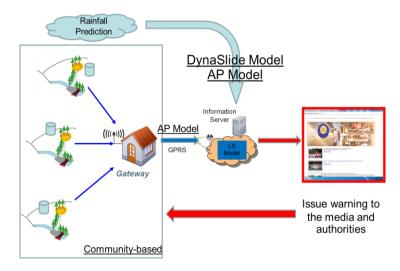
Fig. 6. Multi-way warning system using AP Model
