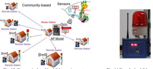
Fig. 13. Community based landslide warning system
